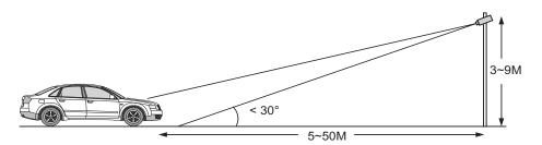
Installing the camera on the side: Install the camera in the side front of
