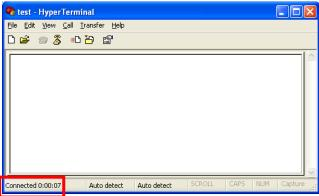
9. Key in items form Cash Register, if the connection established, transaction data would appear as strings in the HyperTerminal box as below figure.
