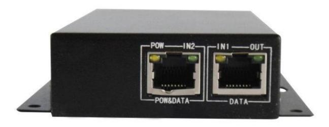
The POE-AT1 is a single-port Power over Ethernet midspan injector that is complaint with IEEE 802.3AT Ethernet standard. The POE-AT1 provides 30 watts PoE. The power supply that is included with this mid-span requires 100VAC ~ 240VAC input voltage, so it can be used for US and European power supplies.
