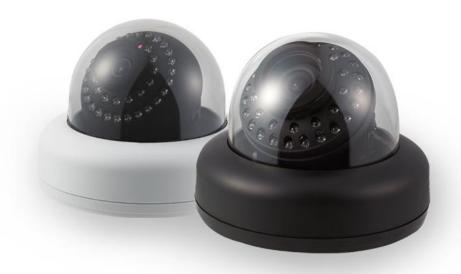
The DPRO-9620VF is an indoor IR dome CCTV camera that is available in a black or white base. The 1/3" Sony Super HAD CCD II image sensor in this camera supports **700 TV lines of resolution in color** (day mode) and **B&W** night mode (low light and zero light infrared).
