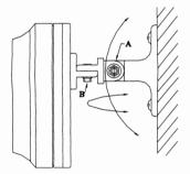
3: Adjust the vertical and horizontal angles by loosening screws (A&B) and by turning the bracket vertically and horizontally.
