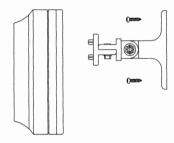
3. Attach the camera case to the bracket.
