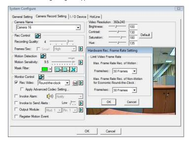
7. Set the maximum frame rate for motion and non-motion periods so as to save as much disk space as possible.
