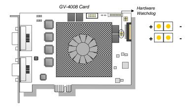
**Note**: To locate the motherboard's Reset (+) pin and the (-) pin, please refer to the motherboard's user manual.
