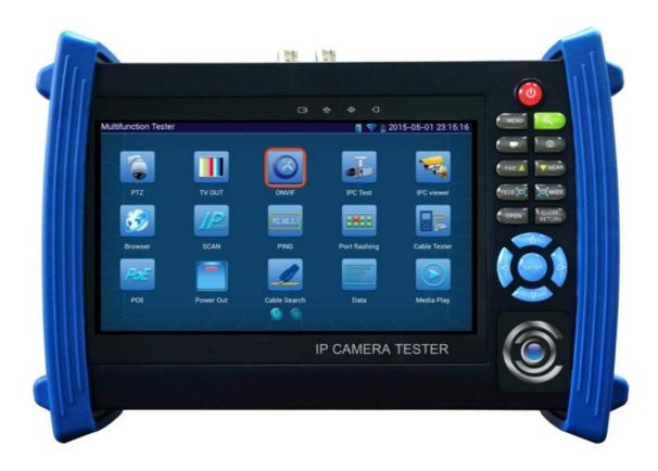
The MON-7HD is an HD CCTV and IP camera test monitor with a 7 inch LCD touch screen. This video tester is capable of displaying video from IP cameras HD CCTV cameras (HD-TVI, HD-CVI, AHD, HD-SDI), and analog CCTV cameras. The  $7^{"}$  LCD monitor supports  $1024 \times 600$  resolution. This is the ultimate testing tool for installers that work with various types of security cameras.
