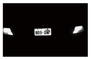
• For **1.3M image resolution**, the captured vehicle should occupy approximately half to two third of the image width.
