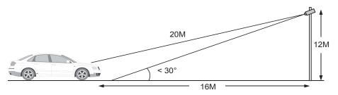
• Install the camera to the front of the vehicle (Recommended)
