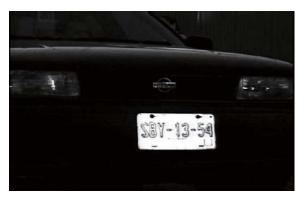
• The plate is in shadow: avoid placing the camera where it is subjected to direct sunlight, reflections or shadows. Recognition may be degraded.
