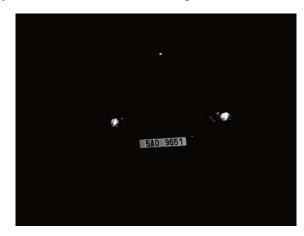
**Note:** The captured plate should be 30 to 35 pixels in height. To check the height, copy and paste the characters into a Paint file and save it in BMP format (e.g. **01-0-8613**). Right-click the BMP file, select **Properties** and click the **Summary** tab to find the Height information.
