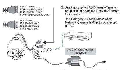
3. Connect the power cable from the Network Camera to a power outlet.
