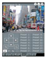
PTZ Control includes full set of tools for remotely steering of PTZ domes. Operator can manually steer in all directions or he can use available presets from a list in order for quick transfer to positions programmed earlier. On manual steering it is possible to choose one out of three speed reactions of PTZ dome which is useful on connections with low bandwidth. Additionally manual Zoom +/- option helps with precise tuning of the dome.
