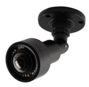
The AHD-BL25 is a wide angle security camera with builtin infrared night vision. The 2.5mm lens captures a 180degree horizontal angle of view (170-degree effective range).
