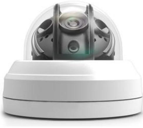
The AHD-D7W is a 1080p resolution HD surveillance camera (AHD CCTV type). This HD camera features a compact indoor rated enclosure. This camera has a **fixed 3.6mm** lens (for a wide angle of view) and a 1/2.9" Sony CMOS sensor which supports **full HD - 1080p video resolution** in both Color (day) & B&W (night) modes.
