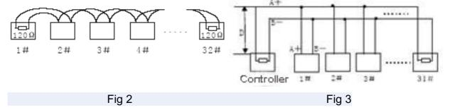
2.2  $120\Omega$  terminal resistance is connected as shown in fig 2.
