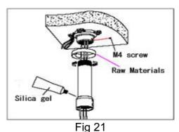
**Note**: If the dome is used in the outdoor conditions, after using enough raw materials to wrap the thread at the upper end of boom, tighten the boom on the base of ceiling. Use the silica gel around the joint sleeve and connector of the boom to be sure water proof
