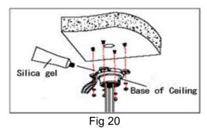
**Note**: If the dome is used in the outdoor conditions, use the silica gel on the faying surface of the base of hang ceiling and the ceiling board and around the out-holes to be sure water proof
