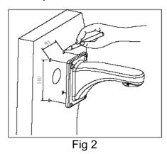
b. As shown in fig 3, fix the wall hanging bracket on the wall with wire and cable through it.
