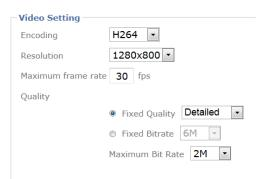
**Resolution-** Here you define the video resolution for the profile. Which choices you have depend on your camera model. Some HD models offer image resolutions of up to 1920  $\times$  1080 pixels whereas standard definition cameras are limited to 640  $\times$  480 pixels.
