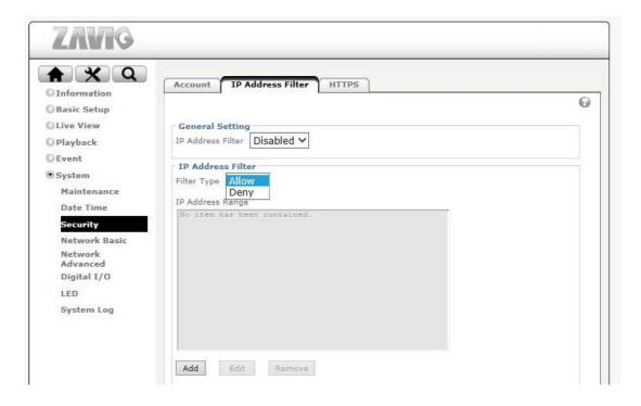
Once you enabled it, the listed IP address are allowed or denied access to the network camera. Add the IP address that you'd like to allow or deny, select allow or deny from the list and save it.
