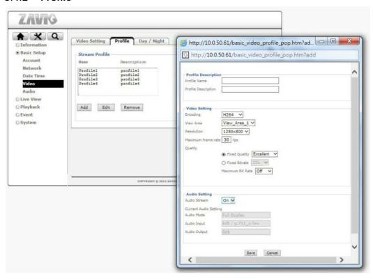
The ZAVIO network camera allows the creation of video streaming profiles. For each profile you can define the video resolution, the viewing area and the video codec that is to be used. Click "Add" to create a new profile, "Remove" to delete a profile or "Edit" to modify an existing profile.
