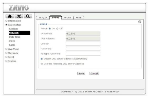
PPPoE is the most common form of connection for DSL-based Internet service.
