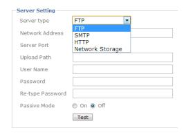
Passive Mode- Select "On" if your FTP server utilizes passive FTP, which is the most common method.
