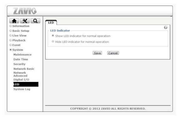
You can enable or disable the operation LEDs on your ZAVIO network camera. Hiding the LED indicator will make the camera appear to be offline while in fact it is operational and captures video.
