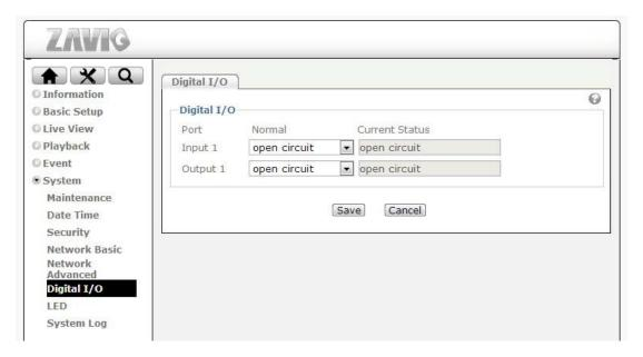
If your ZAVIO network camera is equipped with a digital I/O interface, you can configure the connections on this page. The screen shows the current status of input 1 and output 1. The screen also allows you to define the "normal" state of the port. The normal state can be viewed as the "non-alert-state."
