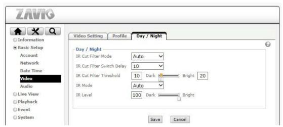
Some ZAVIO network cameras are equipped with active IR LEDs providing the ability to capture video in complete darkness. Note, that if your camera is not equipped with IR LEDs, this menu will not be available. Also note that some menu items will vary depending on your camera model.
