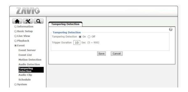
If the image of the camera is obstructed, e.g., because someone covers up the lens or moves the image out of focus, the camera notices this and generates a trigger alert. You can define how long you want the alert state to remain active after the event has occurred.
