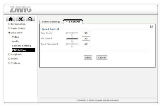
**Speed Control:** With higher speed, the camera would move faster.
