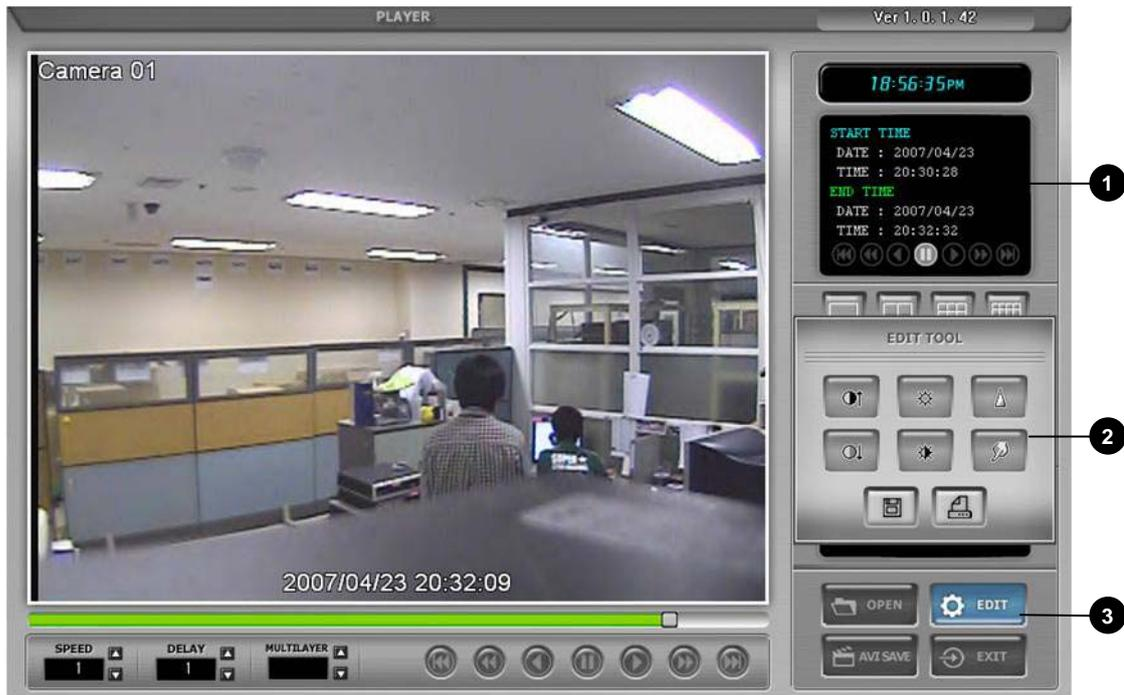
**1** 1. **RECORDED DATA DISPLAY** : Displays start time & end time of recorded data. Also, displays operating status during playback.
