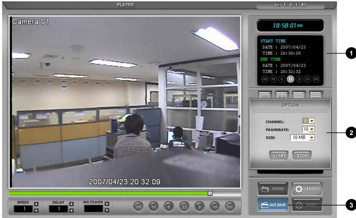
1. **RECORDED DATA DISPLAY** : Displays start time & end time of recorded data. Also, displays operating status during playback.
