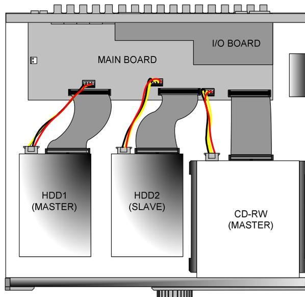
1. Connect Main Board and HDD1 using IDE cable and HDD power cable.
