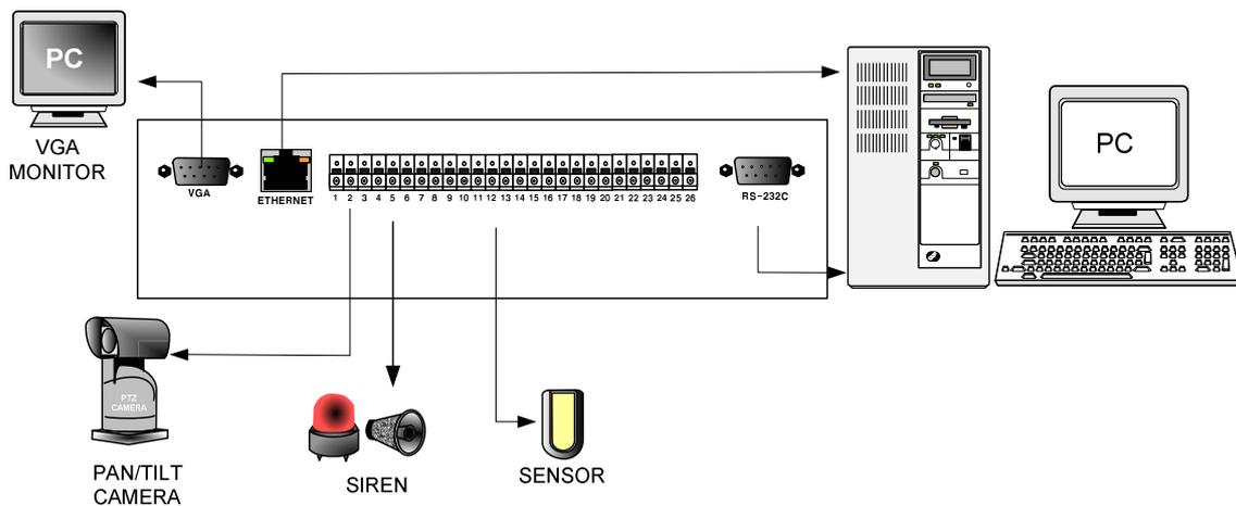
**RS-232C** : Control DVR through RS-232C port by using PC.
