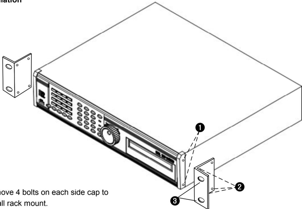
1. Remove 4 bolts on each side cap to install rack mount.
