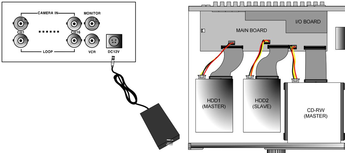
Connect one DC 12V, 8.3 A Adaptor to the back side of Power Jack for right operation of 2HDDs and CDRW.
