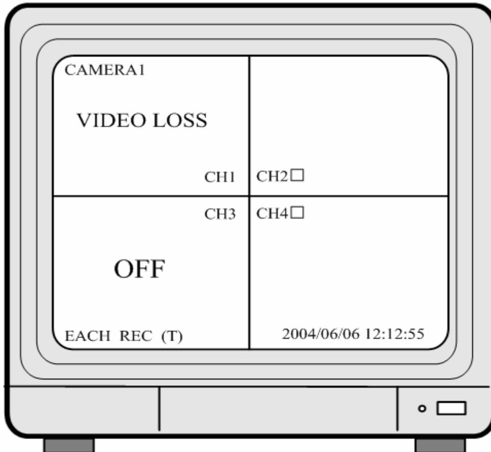
**Note:** CH1: No block figure next to CH1 indicates that it is not recording.
