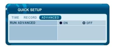
Select "ON" or "OFF" by pressing "-/+" buttons on the remote controller or on the unit.
