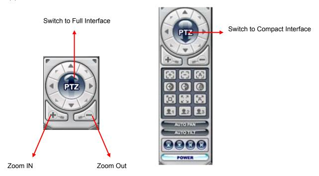
If one or more Pan/Tilt/Zoom Cameras are installed on the DVR, they can be individually selected and controlled using the PTZ control box. To control a channel-specific PTZ camera, simply click on the channel where the PTZ camera is connected.
