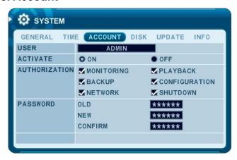
Admin can define each user's Authority. Select User 1~5, then select Activate option **on** or **off**. When enabled, it will be possible to check individually under user settings: Monitoring, Playback, Back up, Network, Configuration (Main Menu Setup), Shutdown (Power off).
