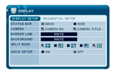
Press [DISPLAY] buttons to activate the multi-screen display. It is changed the order as shown below among your choice of SPLIT MODE. While in 16-way screen display, press [DISPLAY] buttons for 1second to begin full screen sequencing. The sequence mode and dwell times are programmable. For detailed information about configuring those, see "Sequence Setup". If the sequence mode is not activated, it moves to Quad mode instead of Sequencing.
