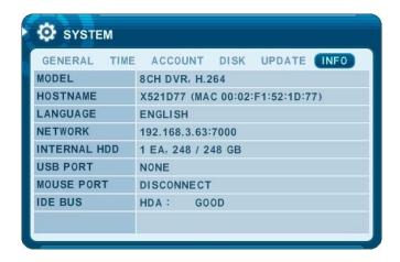
Press info button on IR remote to display the information. The other menu is blocked to move. This menu provides information such as listed below.
