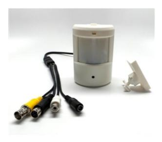
The **AHD-PIR18** is an HD spy camera hidden in a PIR motion sensor housing, allowing the user to discreetly mount this camera indoors. It supports AHD, HD-TVI, and HDCVI HD 1080p modes. The Infrared LEDs featured on this camera are completely invisible, and do not emit a red glow like traditional LEDs. The **940nm IR LEDs** are hidden behind the PIR sensor window, making the camera completely covert when the LEDs are on.
