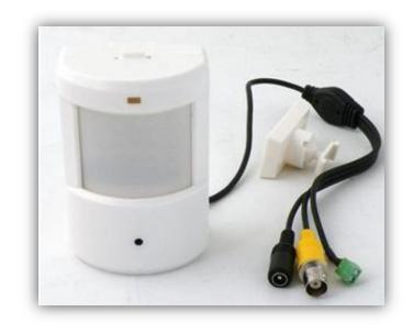
The PIR-IR60 is a high resolution covert CCTV camera that supports **700 TV lines of resolution**. This spy camera provides an incredible color picture in day mode and clear back and white in night mode. The camera comes with a **fixed 3.7mm Lens**, which provides the user with an approximate **86° viewing angle**. The PIR-IR60 hidden IR spy camera is typically used in covert surveillance systems.
