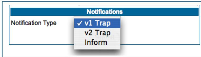
The **Notification Type** pull-down menu allows you to configure the type of SNMP notifications that will be generated:
