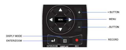
Once "**Default**" is chosen, press "**Enter**" on the remote to return to the main menu. Then using the arrows on the remote to highlight "**System**", then "**Enter**" to select it.
