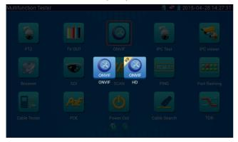
If you select ONVIF SD or HD mode, the meter automatically scans different network segments for ONVIF cameras. It lists the camera name and IP address on the Device List. If no cameras appear under the device list, try clicking on the Refresh button
