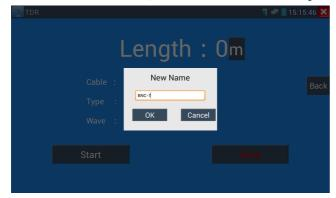
**Application:**TDR test is the use of pulse reflection method, to transmit pulse signal for tested cable, when cable is disconnected or short-circuit, reflected pulse is generated, the tester receives and deals with the reflected wave, measurement results displayed on the screen. TDR cable test can test cable
