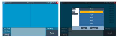
Click "Setting" to choose the baud rate of RS485/RS232; it must be the same as the DVR or the Control keyboard. The DVR or Control keyboard send the code to the tester, if it can be read, the protocol will shown on the upper right, like Pelco D, if not, like P:---
