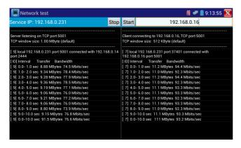
Network bandwidth testing can also be tested with a computer using compatible network bandwidth testing software. Install network bandwidth testing software on a computer, as a test Client or Server, to do the mutual testing with the tester. If use computer as the server, the computer IP address is: 192.168.0.89
