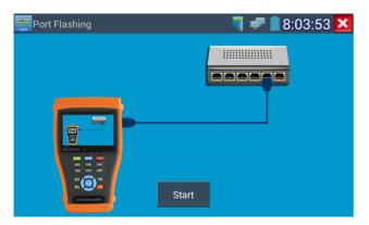
If the tester and PoE switch are connected well, the LAN port of POE switch flash at special frequency, If not, no any changes on the LAN port
