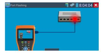
will enable the installers to easily and quickly find the connected Ethernet cable. This function can prevent mistakenly insertion or disconnection non-corresponding cable to artificially interrupt network connection.
