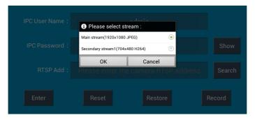
Note: in the event the ip tester does not auto detect the rtsp stream, refer to the specific camera manufacturer for the specific rtsp stream url. you may find this on line with a search of the camera model number and the word rtsp
