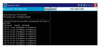
corner of the screen. This app is used to send packets for network speed testing. Click the "Start" button to send the packets and start testing.
