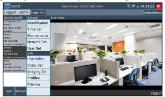
**ONVIF PTZ control:** Tap the image in the direction you want the PTZ camera to move. Tap the left side of the image to move left, right to go right, up to go up and down to go down. Compatible IP PTZ cameras will rotate accordingly. PTZ rotation direction is displayed on top left corner of the image.
