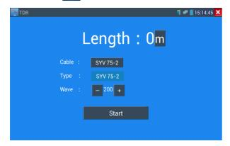
cable type for testing, click "+" and "-" to adjust cable's wave speed .
