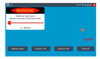
VFL four status can select——"Steady mode", "Evasive 1Hz", "Evasive 2Hz"and "Time off". Click button "Steady mode" to enter steady status, click button "Evasive 1Hz" and "Evasive 2Hz, to enter pulse mode, click button "Time off", VFL be turned off. Timed turn off can select (5mins, 10mins,
