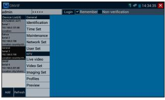
**Live Video:** Click "Live Video" to view the live video feed from the IP camera. To make the image full screen, double tap on the video. Stretch two fingers outward or inward on the touch screen to zoom the image in or out.
