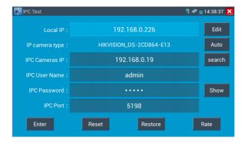
IP Camera's IP: Enter the IP camera's IP address manually or click "Search" to auto-scan for the IP camera's IP address. It is better to directly connect the IP camera to the tester so the search results will only display the camera's IP address. If the tester is connected to a PoE switch, it will find and display several IP address
