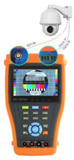
(1) Connect the SDI camera's video output to the IP tester's "SDI IN" interface, the image will display
