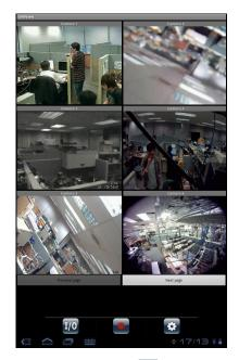
I/O Trigger **1**/0: Forces I/O devices to be triggered.
