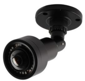
The HD-TVI-BL180 is a 180-degree HD-TVI camera with built-in infrared night vision. The 2.5mm lens captures a 180-degree horizontal angle of view (170-degree effective range).
