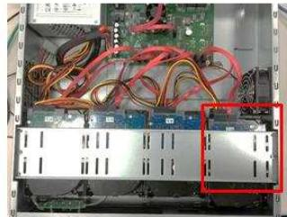
3. Assemble the HDD bracket back to the cabinet and insert the SATA cables and power cable.
