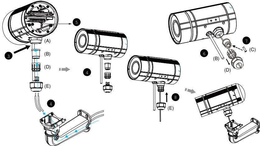
4. You may choose to use AC24V or DC12V inputs as power source, please feed the power lines through the wall mount bracket and the waterproof connector (E → D → B → A) as illustrated below. Pass power lines through the rubber seal (B) and then connect the power lines to the terminal block.
