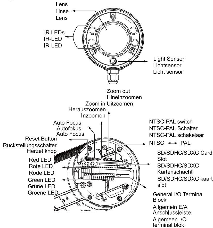
**3****Hardware Installation / Hardwareinstallation / Hardware installeren**
