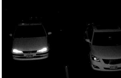
Clear Image Captured with IR Illuminators and Headlight Filter
