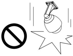
● Do not manually pan and tilt the Network Camera when the power is on.
