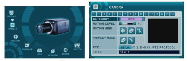
1. Press Left/Right buttons [ \* ] or number button to select the desired camera
