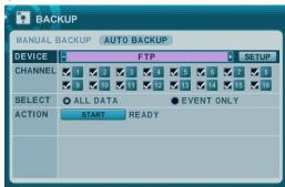
2. Use direction button to move FTP setup. The menus are displayed with options on the left-hand column and settings in the right hand column.
