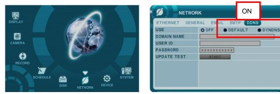
The menus are displayed with options on the left-hand column and settings in the right hand column. A cursor (highlighted menu) can be moved using the Direction buttons  $[\overset{\bullet}{\phantom{\bullet}}\overset{\bullet}{\phantom{\bullet}}]$ .
