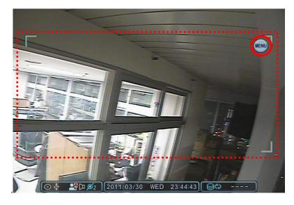
4) Press menu button to have the virtual PTZ controller. Zoom in/out,Go to, Tour and other function can be controlled by using the virtual PTZ controller.
